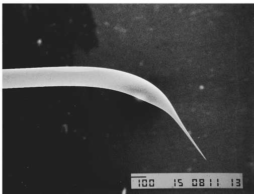
FIG. 3. A representative scanning electron microscope image of the probe made from an optical fiber coated with aluminum.
